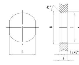
Installation direction: o-ring sits on chamfer.
